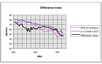
The third plot is a comparison of the estimated level and the actual level of emissions from the EUT. To calculate the signal which caused the field to rise from level XdBuV/m to level YdBuV/m we cannot simply subtract the to numbers to find the difference.
