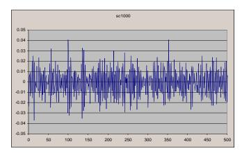
Plot sc1000 shows the two sources radiating simultaneously. The frequency of the impulsive spikes has increased, in fact doubled, but the peak levels are unaffected.
