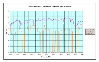
Then plots were taken with first one then both sources switched on. The plot shows the results. The difference trace includes intermittent excursions to minus infinity where the calculation attempts to find the log of zero! The cause of this little difficulty is at frequencies where the ambient result and the ambient + EUT result are the same (or negative).
