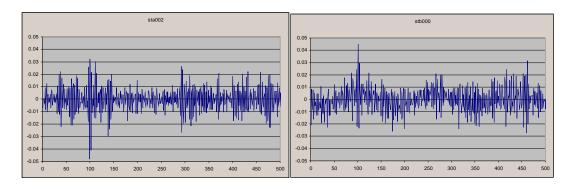
Plots sta002 and stb000 show the signal from the antenna with each source switched on independently. The impulsive nature of these sources is immediately evident. Fourier analysis shows that for a flat (ish) spectrum in the frequency domain, the time domain must have a transient nature. The signals are completely random in nature, as expected from noise sources.
